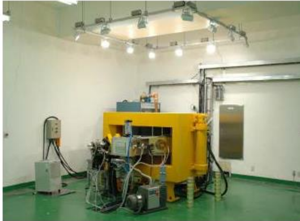
Fig. 1: A 13 MeV cyclotron (indigenous product) in operation in Chosun University, Republic of Korea.
