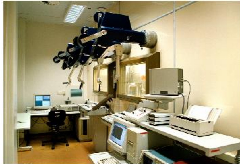
FIG. 2 Hot cells with manipulators used for radioisotopes/radiopharmaceuticals production available from commercial sources.
